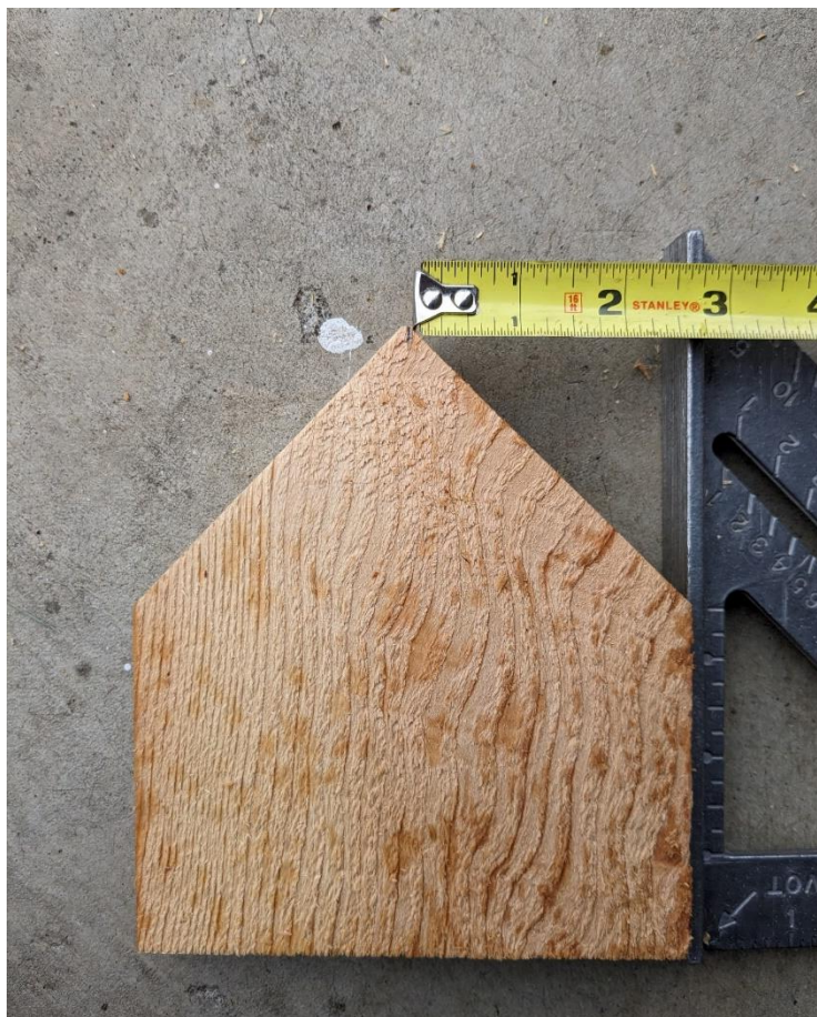
Figure 5 - Cut the back board at 45 degrees from center
