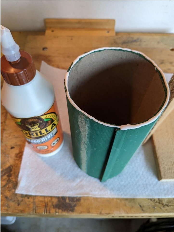
Figure 18 - Apply glue to rim first, then quickly to the side of the tube
