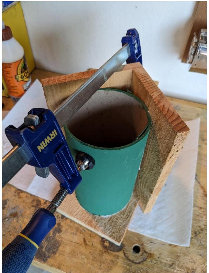
Figure 19 - Quickly set the tube in place and clamp the tube to the roof
