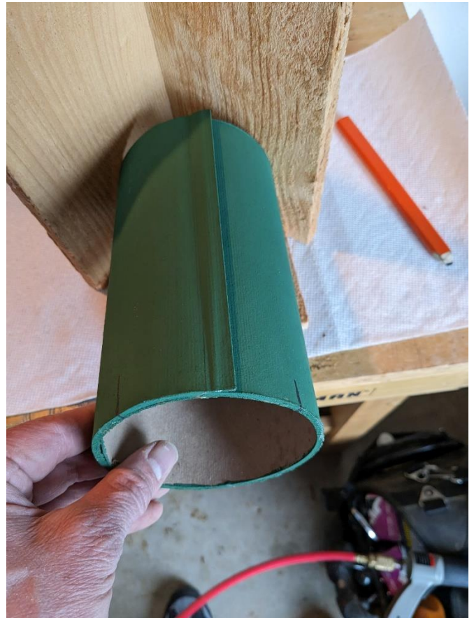
Figure 15 - Marked tube, ready for sanding
