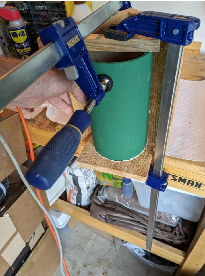
Figure 20 - Use a wooden cleat to help clamp the tube to the back
